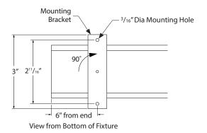
Step 2: Mount fixture(s) (means of mounting and mounting hardware by others\*) \* Consult factory for ceiling or wall pocket mounting information.
